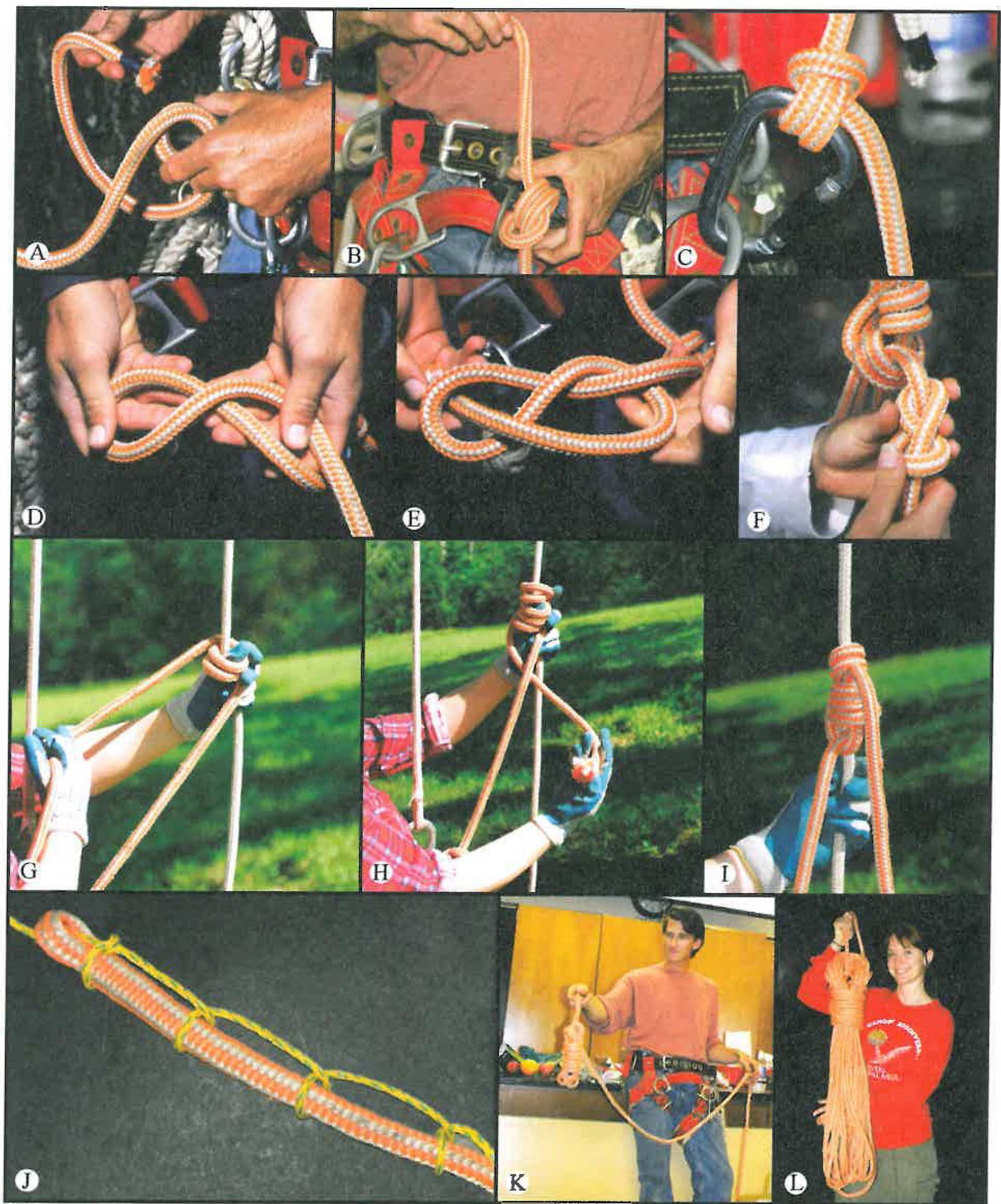
FIG. 6. A–L. Climbing knots. A–C. Anchor Hitch knot. A. Pass the working end of the rope forward over and through the carabineer twice forming two loose turns moving left to right. B. Pass the working end across the two loops from right to left then through the two loops from left to right. C. Tighten and dress the knot and add a figure eight stopper knot. D–F. Figure Eight stopper knot. D. Form the working end of the rope into a loop. Cross the working end over and under the running end forming another loop. E. Pass the working end through the first loop from the front. F. Tighten and dress the knot. G–I. Blake's Hitch Knot. G. Grab working end of rope with left hand. Use left thumb as a spacer and make four to five counter clockwise upward turns with first two or three turns over thumb. Make sure bridge between saddle and Blake's Hitch is not too long or too short. The bridge needs to be a comfortable length in a sitting position, ensure that the extra give from the climbing saddle does not lengthen the bridge to the point that the Blake's Hitch is out of reach. H. Pass the end of the split tail behind turns. Then pass the end of the split tail between bridge and working end of rope. I. Pass the end of the split tail through the lower two or three turns (depending on whether four or five total turns) held by thumb. Dress and set the knot and add a figure eight stopper knot (see F). J. Half Hitch. Pass the end of the throwline around the end of the climbing rope in a clockwise motion. Pass end of throwline over climbing rope and under throwline. Repeat Half Hitch four to five times moving down the climbing rope away from the end of rope. K. Monkey Fist. Coil 3–5 m of working end of rope. Cover the coils with several turns of rope. At end of turns form a loop and pass it through one of the loops formed by the coils. L. Gasket Hitch. Coil all but the last three to five feet of rope. While holding onto coil with one hand, make clockwise horizontal turns around the coil moving towards the head of the coil. Push a bight through and then over the head of the coil and slide bight over coil until it rests on top of the turns. Pull the end of the rope to tighten and set the knot.
